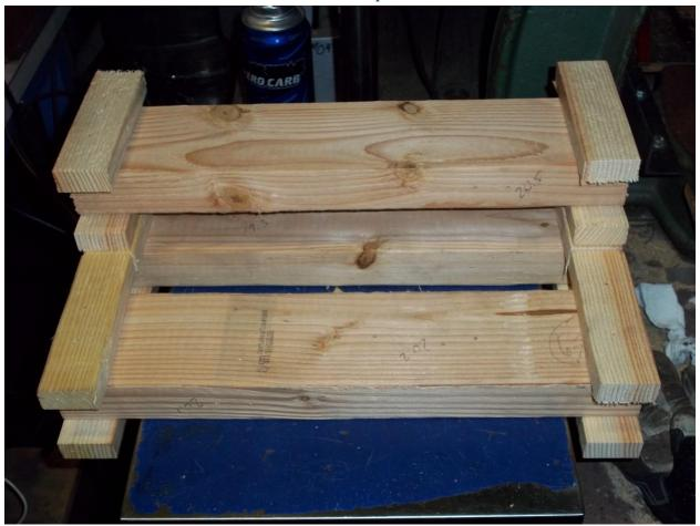
Fuel consisted of 2"x4"x16" Green, Douglas fir. Detailed fuel load specifications for each run can be found in the corresponding digital folders submitted with this report.
