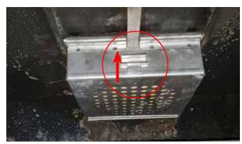
8. Pull the flame shield forward and tilt down, be prepared to support catalyst assembly
