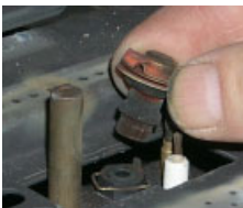
Remove the 2 screws, push Burner Assembly to the left and lift out.
