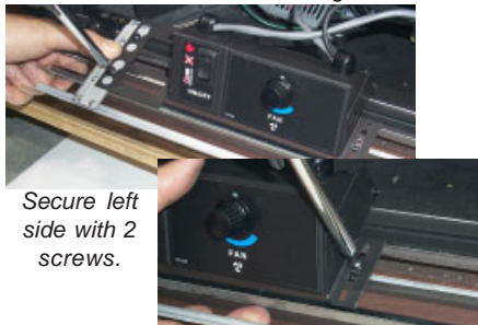
Secure right side with one screw.
