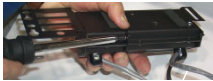
Secure the 2 boxes together with one screw.
