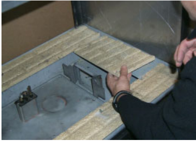
Remove Left & Right Side Base Brick Panels
