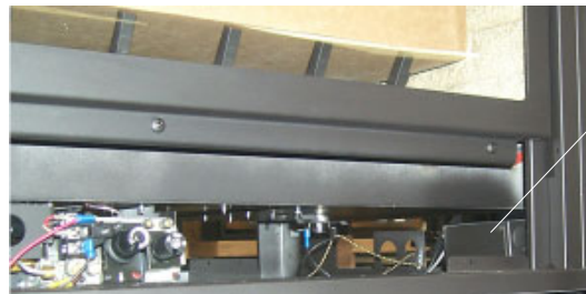
Remove cover to access Terminal Block
