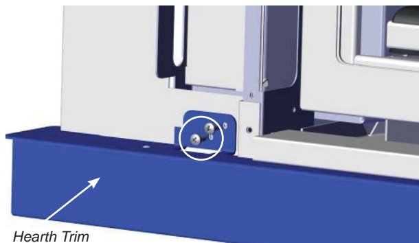
Diagram 3—Hearth Trim Secured to Backing Plate
