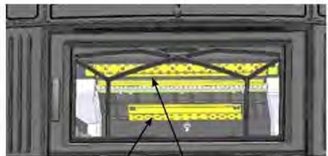
B- Combustor Flame Shield - loosen 2 x 7/16" bolts to remove. E- Bottom Shield
