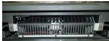
Secure fan with 2 screws removed in Step 1
