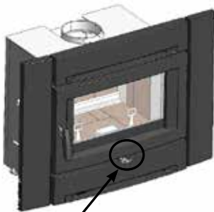
Primary Air Damper Left - Open Right - Closed
