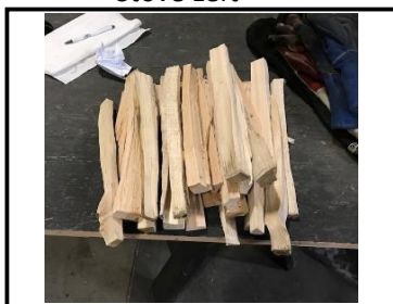
Typical Start-up Load
