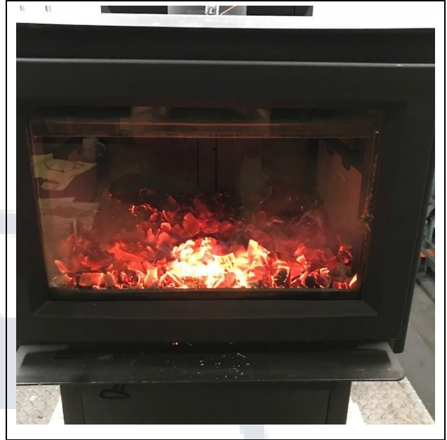
Residual High Fire Load Coal Bed
