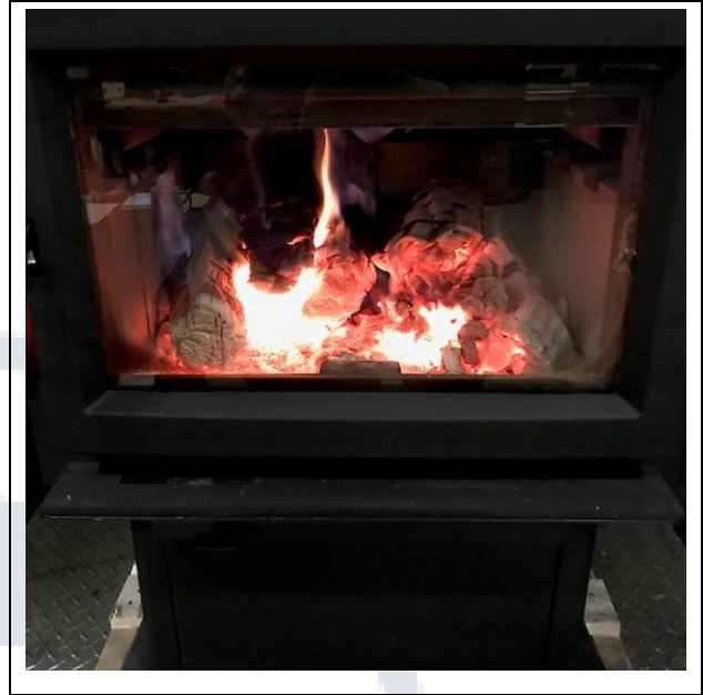
Residual High Fire Load Coal Bed
