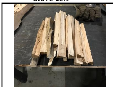
Typical Start-up Load
