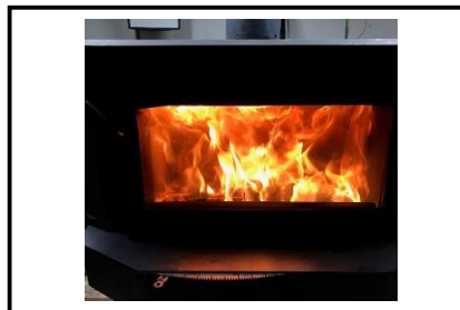
Typical High Fire Coal Bed
