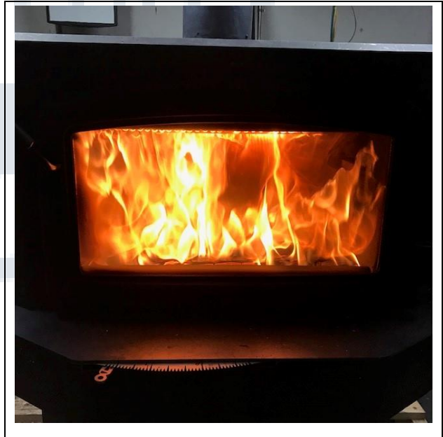
Residual Start-up Fuel Coal Bed
