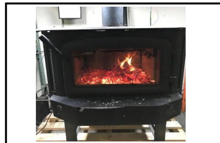
Typical Low Fire Coal Bed
