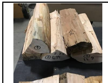
Typical Low/Med Fire Load
