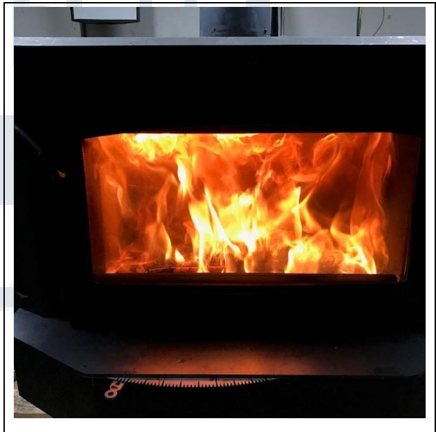
Residual Start-up Fuel Coal Bed
